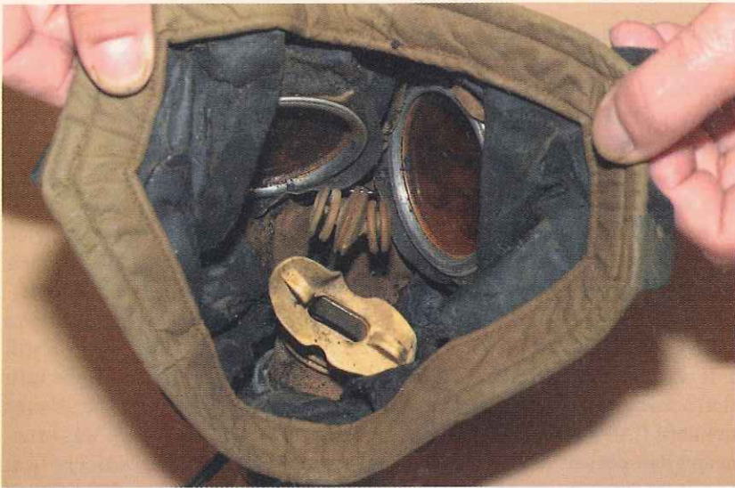
The small box respirator and its haversack. This unit replaced the earlier, less effective P and PH gas helmets. The rubberized face mask contained protective lenses, nose clips and a rubber mouthpiece. Filtering was done through activated charcoal.
