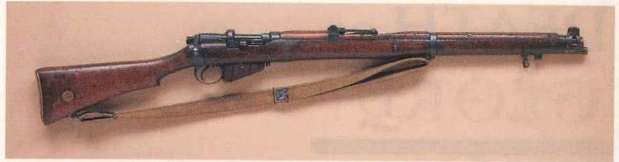
The primary British Battle rifle of the Great War was the Mark III Short Magazine Lee Enfield. One of the finest battle rifles of all time, the SMLE's magazine held 10 rounds of .303 ammunition. It was rugged, reliable and accurate. The same pattern was issued to infantry and cavalry.
